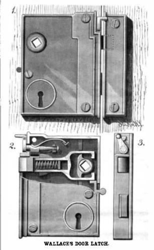
Fig. 1 in the engraving shows the lock in side elevation. In Fig. 2 a portion of the casing is broken away to show internal parts, and Fig. 3 is an end view.
