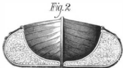
TRANSVERSE SECTION OF LIFE RAFT.
