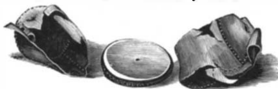
FRAGMENTS OF THE EXPLODED BOILER.
