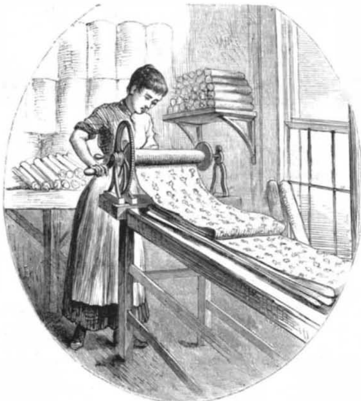
THE MANUFACTURE OF WALL PAPERS.—WINDING IT INTO ROLLS.
