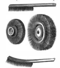
Where the article is to receive a deposit of gold or silver are usually made of brass or steel wire, and of a variety of its surface is usually softened by slightly amalgamating it shapes to suit the object. Some of the forms are shown in
