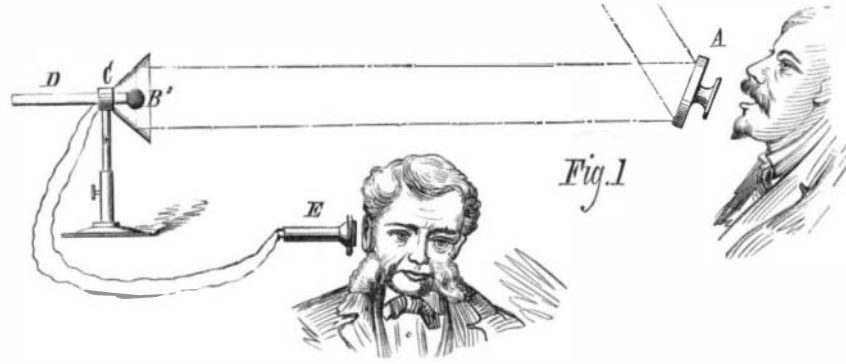
MAGNETIC THERMOPHONE WITH REFLECTING DIAPHRAGM TRANSMITTER.
