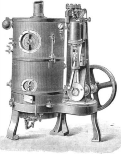
ENGINE WITH GAS-FIRED BOILER.
