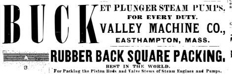
B represents that part of the packing which, when in use, is in contact with the Piston Rod. A the elastic back, which keeps the part B against the rod with sufficient pressure to be steam-tight, and yet creates builtitle friction. This Packing is made in lengths of about 20 feet, and of all sizes from ½ to 2 inches square.
