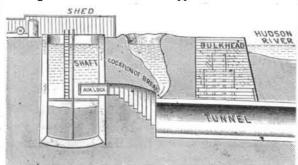
Our diagram shows the place of the accident. The workmen, twenty-eight in number, ran for the air lock chamber, and all would have been saved could they have got in; eight of them had succeeded in entering the lock, when down came the iron roof plates, earth, mud, and water, closing the entrance door to the lock chamber and cutting off the escape of the remaining twenty men, who were quickly suffocated, to help them being impossible.
