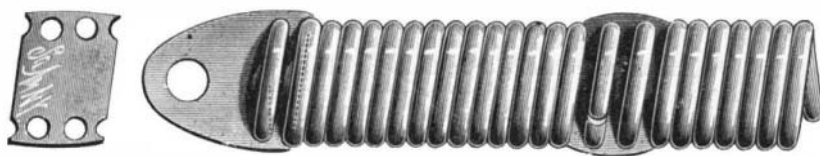
MENDING BROKEN SPIRAL SPRINGS
