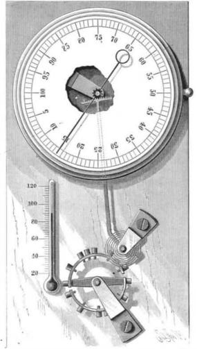
IDE'S APPARATUS FOR ADJUSTING BALANCE WHEELS 0F WATCHES
