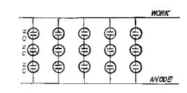
Of course this is equivalent to three large single cells, each exposing five hundred square inches of zinc (equal to a plate about sixteen inches square, exposing both sides). Large batteries of the dipping form, admitting of the immersion of the proper quantity of zinc, are often convenient.
