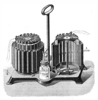
FIG. 1.-THERMO-ELECTRIC BATTERY OF M. NOE
