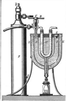
wax, etc. B is a stopcock which is opened and closed part of the methyl chloride that evaporates escapes through the opening, S. As soon as the temperature has fallen to -8° (the boiling point of methyl chloride), the opening, S, is closed. If it is desired to lower the tem-In this way a quart of alcohol can be kept at a temperature of -67° for several hours.
