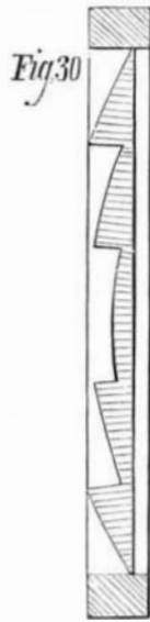
Section of a polygonal Burning Lens.
