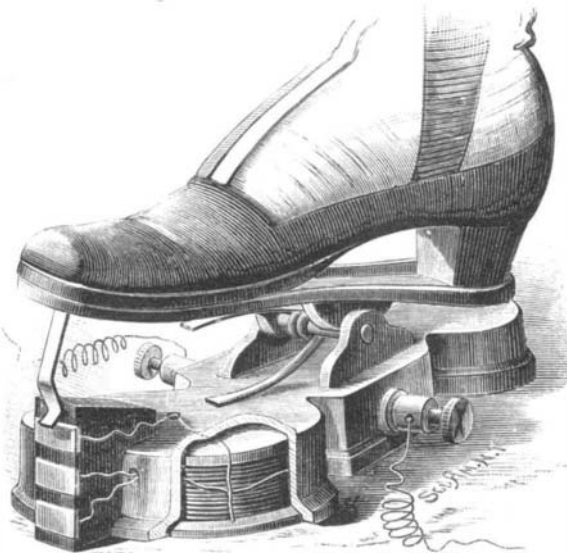
HUSSEY'S SWITCH PEDAL FOR CONTROLLING ELECTRIC MOTORS.
