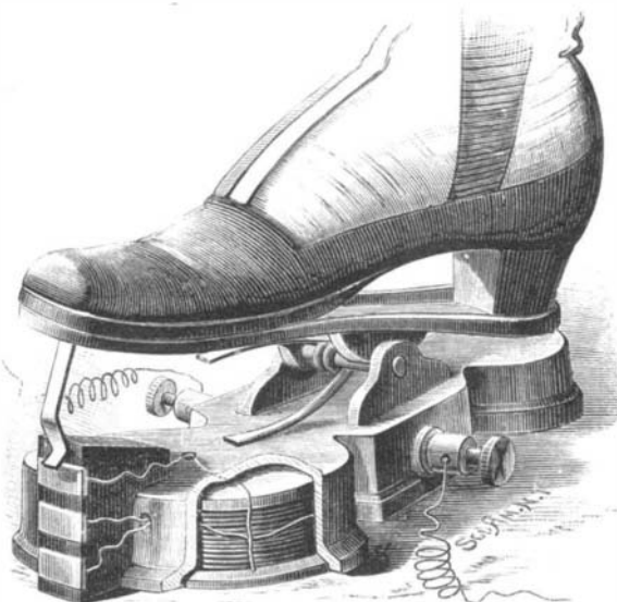
HUSSEY'S SWITCH PEDAL FOR CONTROLLING ELECTRIC MOTORS.
