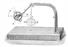
In Fig. 2, A is a brass ring suspended at a, so that it may swing freely around an axis, e.e. Within this ring is suspended a second ring, B, revolving around the axis, b b. T is a circular disk turning with its axis, t t, within the second ring, B; a plane, laid through t t, traverses perpendicularly one laid through b b. At a the ring, A, is
