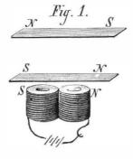
end of the needle and attract the N end; but the polarity of pear. This may be verified by disconnecting the battery, as shown in Fig. 2, when the magnetism remaining in the bar will be found the same as in its first position in Fig. 1.
