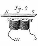
magnets available as a source of power, Mr. Gary absurdly claims to cut off the attraction of the magnet by the use of a thin piece of sheet iron placed on his so-called neutral line; but this is no cut-off. The sheet iron acts simply as an induced magnet of very little power, sufficient, of course, to affect the delicately poised needle placed in its immediatevicinity; but when
