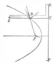
at G oneend of a cord equal in length to E G; fix the other end to the focus, F; slide the square steadily along the straight edge, holding the cord taut against the edge of the square by a pencil, D, and it will describe the curve.
