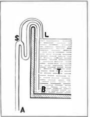
of water is carried from the bottom of thetank. Into the tank, T, is passed the waste pipe, Λ B, of a diameter
