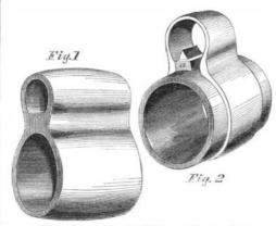
A is the sight protector, as seen when not in use; B is a view of the same position on the barrel of the rifle; C being the sight as shown shaded from the
