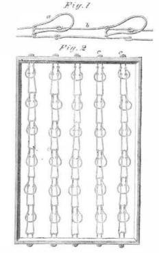
A series of chains, formed of the bent loops, a, and connecting links, b, in the manner plainly shown in fig. 1, are stretched across a rectangular frame from end to end, as represented in fig. 2. The chains are stretched to a proper tension by wedges, cc, at their ends; and they are so arranged that all of the loops will be inclined in the same direction, as shown.
