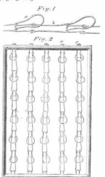
A series of chains, formed of the bent loops, a, and connecting links, b, in the manner plainly shown in fig. 1, are stretched across a rectangular frame from end to end, as represented in fig. 2. The chains are stretched to a proper tension by wedges, cc, at their ends; and they are so arranged that all of the loops will be inclined in the same direction, as shown.
