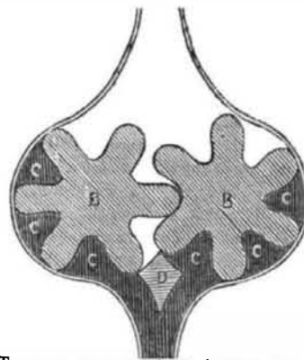
WHEEL ROTARY STEAM ENGINE. FIG. 48.
