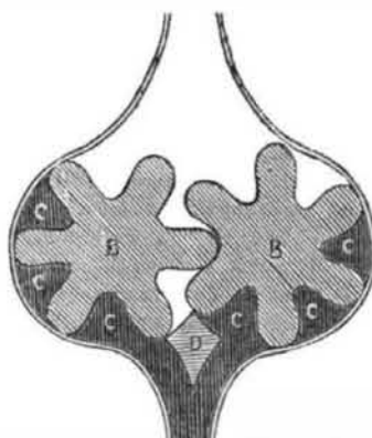
WHEEL ROTARY STEAM ENGINE. FIG. 48.
