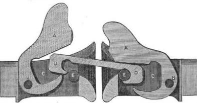
by Mr. Joshua O. Lewis of Worcester, Mass. and it is a good one. This is a longitudinal section showing the inside of the coupling that are made to vibrate on pins B B. D D, is cannot be raised without lifting up A, as patent.
