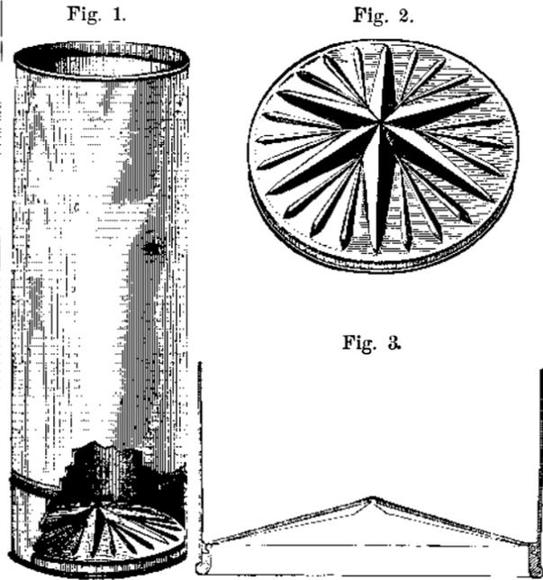
the accompanying engravings a roving can is shown which is calculated to withstand the abuse to which such articles are usually subjected.
