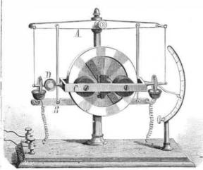
The instrument shown in the engraving should, when the axis of the frame, C, is adjusted equatorially, indicate 15° motion per hour in any latitude. The possible application of this instrument in a larger form to equatorial telescopes in place of the present clock trams, suggests itself. The only difficulty, if any, would be in providing telescope mountings of sufficient delicacy.
