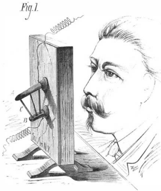
MICROPHONE WITH GRAPHITE RODS.
