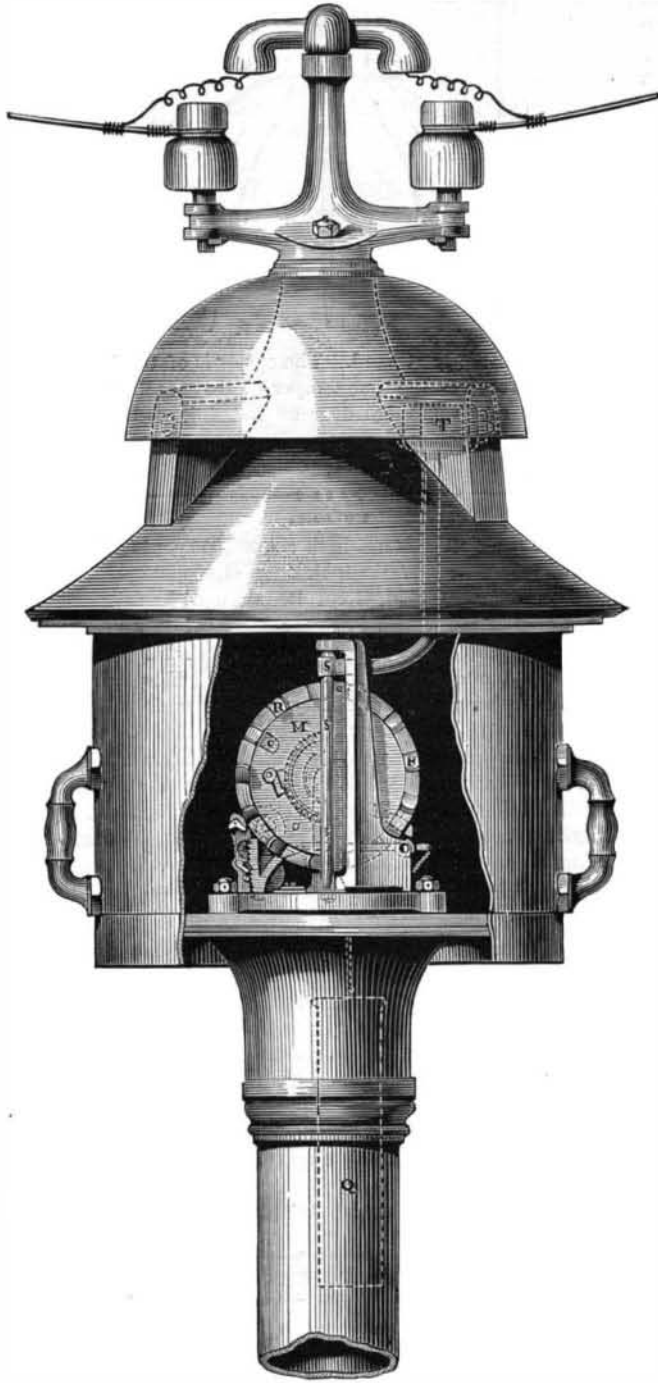
Fig. 4.—FIRE ALARM GONG.
