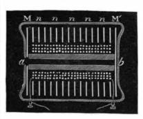
tubular magnet surrounded by a coil of wire. Opposite one pole, a, is a circular membrane, M, similar to that on the ordinary telephone, except that it is pierced with a central hole, the diameter of which equals
