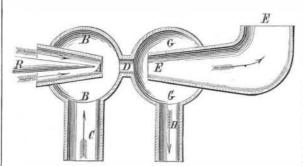
through the diverging "Venturi" tube, E E. If this last be sufficiently "flaring" and the course of the jet unbroken, the water will be able to rise in the tube, E E, to a height (or against a pressure) proportionate to the amount of taper of the diverging cone. If the tube widen, say, from a in section to b, this pressure of the water column will be equal to
