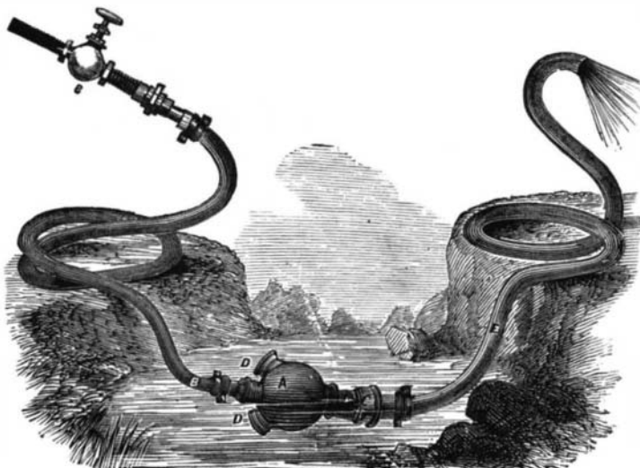
Fig. 2.—PORTABLE RAILWAY STEAM SIPHON PUMP.
