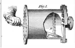
4 and 5. The junk ring was provided with a small tool holder, such as is used upon boring bars. The tool was fastened in the holder while its cutting edge was in the groove referred to, cut as deep and as far up the cylinder as the counterboring was to be. To the junk ring was fastened,
