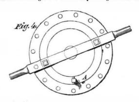
end. This end must then be heated by two long bolts, a wooden lever extending above and across the cylinder. Two men walked around pushing the lever, and when the tool at each revolution arrived at the groove, a fresh cut was taken by moving the engine so as to raise the piston the necessary amount. It is obvious that the piston head may be steadied and held true in the bore of
