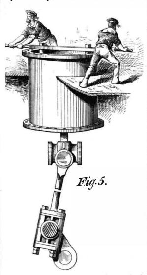
the cylinder by means of a few wooden wedges. Thus we see that in this operation the junk ring was made to serve as a boring bar head, the men furnishing the necessary rotative motion, the feed motion to the tool being obtained by advancing the piston toward the end of the cylinder where the work was being done.
