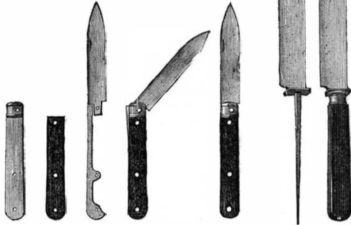
Fig. 2—TABLE AND POCKET KNIVES TAKEN APART.
