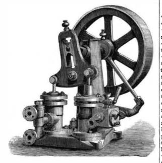
lbs. when the belt pulley is substituted for the fly wheel. When single the capacity of the pump is from 2 to 4 gallons. The apparatus is the invention of Mr. A Schmid, of Zurich, Switzerland. We take our illustration from the Revue Industrielle.
