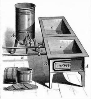
In from twenty to thirty minutes the butter is soft enough to be worked easily by hand with the ladle, the heat of the water bath producing thus about the same effect as the change of temperature from a cold to a warm day. The heat, however, is not sufficient to melt the butter so as to injure the same. Should the bath get too hot, the current of steam or hot water is shut off and conducted into the regulating tank.
