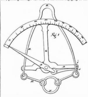
edge of the slot. To the opposite end of the bar, I, is pivoted the pointer, D. G is an arm attached to the bar, B, curved at its upper end, and carrying the indicator, C.
