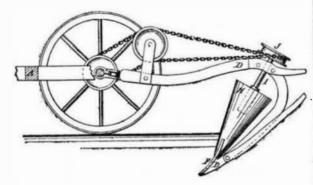
through the Scientific American Patent Agency, May 22, 1877, the novel plow illustrated herewith. The rear parts of the beams, D, are curved forward to serve as standards for the plows, F. From notches in the top of the plow plates
