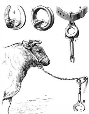
It consists in a crescent-shaped hook, A, and a ring, B. The hook is slipped into the ring, as shown, forming a coupling which can be operated instantly and easily, which already in flames, under the management of Alderman V. cannot be accidentally detached, and which, not being de- Nieswand and Mayor Steinkopf. Fortunately, these gentlependent on any screw or spring, is as strong and durable as the ordinary links of a chain.
