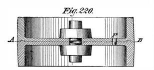
couple of holes may be bored and tapped three eighths or half an inch, or larger if thought necessary, near the rim, diametrically opposite each other.
