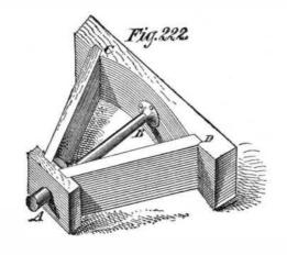
is repeated until the circle of the pulley is finished. Into the mould so prepared mnst now be placed six cores made in the box described in Fig. 222, and also the core to make the hole for the shaft. The whole is then covered with a level cope, and prepared for the casting.
