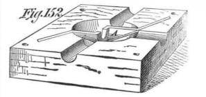
and is on that account more difficult to  $e_X$  tract from the core than if it were straight and vertical. When, however, the partitions are of this curved form, the pieces of which they are formed are composed of metal, brass being generally preferred. Patterns have in this case to be made wherefrom to cast these pieces, and they may be made as follows: First two half pieces, such as shown in Fig. 153, are turned; each
