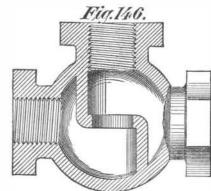
the openings. The flanges vary in shape; but as a rule, small valves are provided with hexagons and large ones with round fianges suitable for bolting to similar fianges to make For small valves, say up to 2 inches, the pattern is joints.
