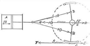
through the medium of the engine frame, upon the center of the driver in the opposite direction. When the crank is below the center of the wheel, the 10 tons acting upon its pin is divided equally, in this case, between the center of the wheel and its tread, 5 tons at each point; but as the 10 tons acting against the head of the cylinder and the center of the wheel in the opposite direction is just double this amount, the impelling force, in the direction of F and C, will of course be 5 tons.
