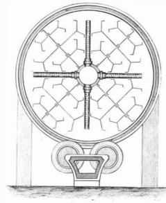
FIG. 5.—COFFEE DRYER, TRANSVERSE SECTION.
