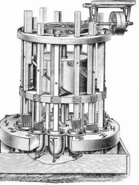
FIG. 6.-GUARDIOLA'S COFFEE HULLING AND POLISHING MACHINE.
