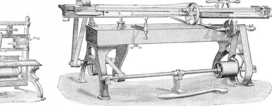
drawing the spoke forward and releasing it from the stop, the desired bevel is given to the edge of the tenon by means of the cutters, the particular inclination being determined by an adjustable angle gauge.
