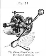
hand power, motion being transmitted to the several parts by means of gearing; the pipe is shown projecting toward the left, and is held stationary by the adjustable jaws of the pipe visc. The pipe passes through the center of the gear wheel, the rotary motion of which is imparted to the die in the die box by means of studs or guides upon which the die box freely slides forward as the die passes upon the pipe.
