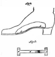
giving great elasticity. A is the spring, which is made of steel, and of such a length as to extend from the heel to, or nearly to, the ball of the foot, and which is bent A, is made with a cross head, B, at each end, as shown in Fig. 2. Through the ends of the crossheads, B, are formed holes, to receive rivets for securing the said spring to the insole of the boot or shoe. The rivets have wide flat
