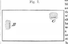
the effect of the blow would be as denoted by the radial lines; while if the position of the hammer face were turned to a right angle, and a blow were struck with the hammer travel-
