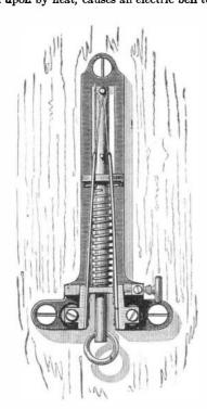
which may ordinarily be employed in lieu of the common press button. In houses and hotels where electric bells are altogether used for purposes of communication, this little device provides a fire alarm wherever a bell-button is located, the locality of the fire being, of course, indicated by the prolonged ringing of the bell.
