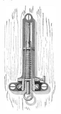
angle. The more dilatable metal being thus placed outside, the tendency of the plates on becoming heated is to curve inward, and thus contact is established at the summit of the angle, the current passes, and the gong, elsewhere located, sounds.
